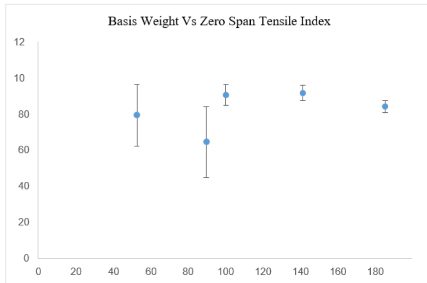
Figure 3.20: Zero span test of spray coated sheet prepared by different concentration of CNF. Influence of Velocity of the conveyor:
