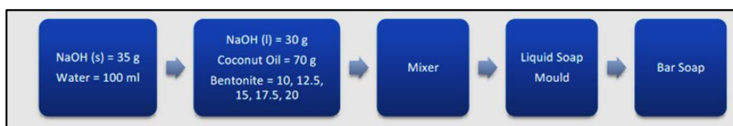
Figure 5.1: Flow diagram of the process of making bentonite bar soap
