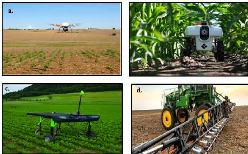
Figure 9.23: Smart robots and mechanical implements for SSWM a. Quadrocopter UAV b. Terrasentia weeding robot c. Ecorobotix d. Weed Seeker
