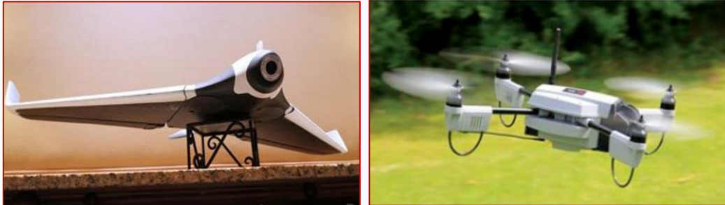
Figure 1.4: Fixed wing and multi rotor type of drones.
