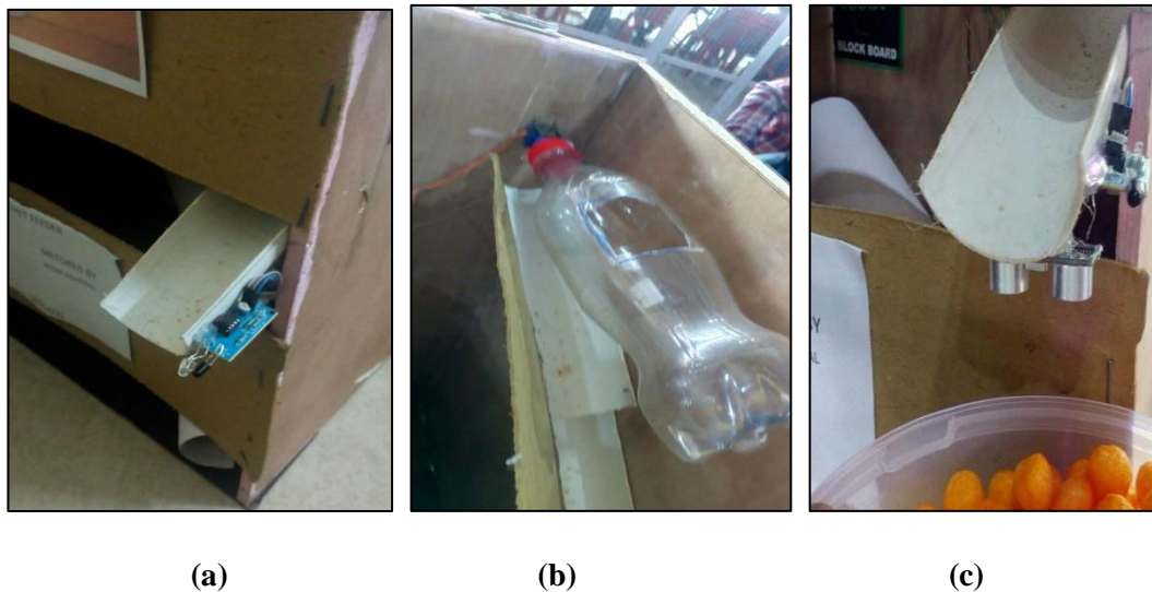
Figure 11.4: (a) IR Sensor attached to pet feeder (b) Bottle (feeder) attached to servo motor (c) Ultra Sonic attached to pet feeder
