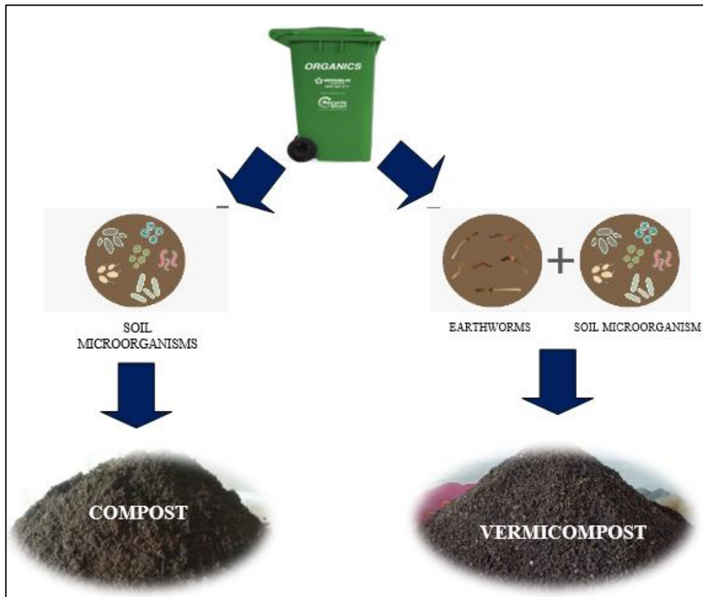
Figure 3.2: Conversion of organic waste into compost and vermicompost
