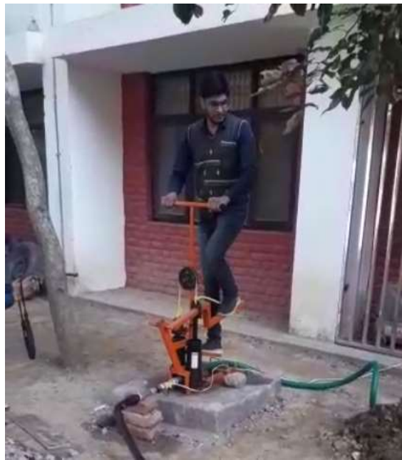
Figure.2.8 Treadle Pump Installed on Concrete Base
