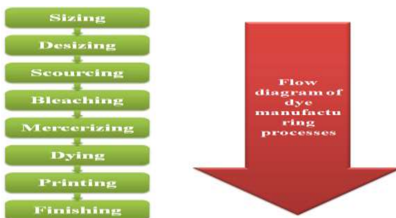
Fig.10.1. Flow diagram of textile manufacturing processes [1]
