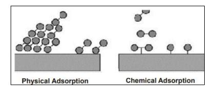
The distinction between chemical and physical adsorption [6]
