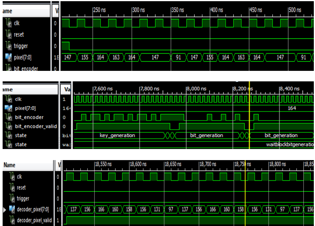
Figure 3.12: HDL simulation result of image (512×512) encoder: (a) Pixel from block memory; (b) Huffman coded bit stream along with 20-bit modulation key; (c) Decoded pixel
